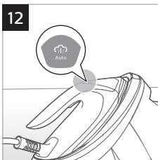
Your appliance comes with intelligent automatic steam thanks to DynamiQ sensor technology which recognizes how and when your iron is moving. When you turn on your appliance, this mode will be activated by default (Fig. 12). Coupled with ActiveSense technology, your iron will steam automatically the right amount of steam based on your movements and the fabric type without the need to use the steam trigger.
