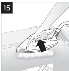
*Note: For best result on tough fabrics such as cotton, linen and denim, keep the steam trigger pressed continuously when you move the iron over the fabric (Fig. 15). Then move the iron over the same area a few more times without steam to dry the fabric.*
